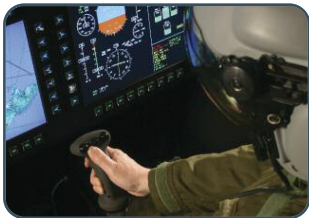
Ultra provides advanced, multi-function pilot's stick-tops for 'flying' uninhabited air vehicles
