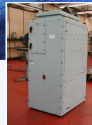
Lubricating oil pump power supply
